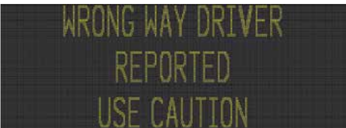
Figure 37. DMS Messaging for WWD Alert (Courtesy of WisDOT)
