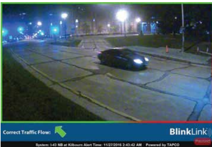
Figure 36. WWD Video Verification (Courtesy of WisDOT)
